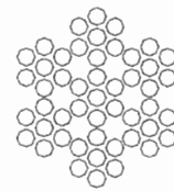
FIGURE 51. Type VI, small cords, class 2, 7 by 7.
